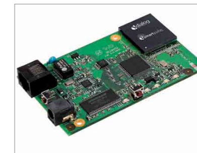
SmartPulse reference design and dev kits enable rapid development of remotely managed home automation systems
