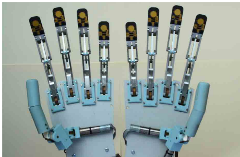
Figure 1: Southampton hands. Across each palm can be seen a dc motor with a worm and wheel to rotate the thumb. Five other motors flex and extend the fingers and thumb. The fingertips have touch (force), slip/texture, and temperature sensors.
