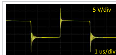
Figure 2: Stray Inductance Associated With Board Traces and Component Leads
