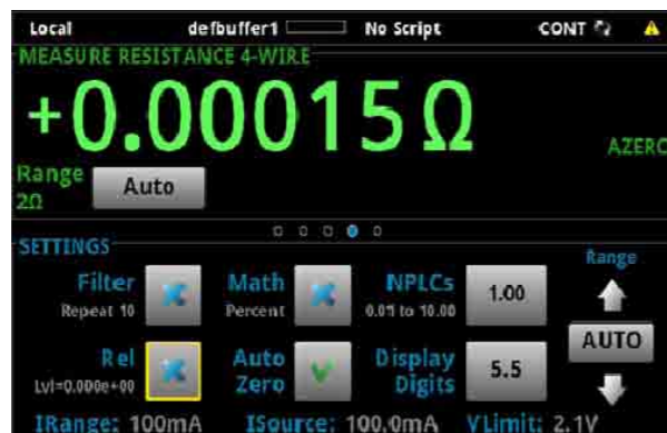
Figure 4: All the controls needed to configure a measurement function are accessible through the same screen
