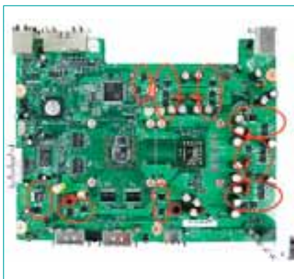
Figure 1. Photo of the Xbox 360 motherboard, showing the CPU and GPU chips being literally surrounded by D-Pak MOSFETs that are supplying their power.
