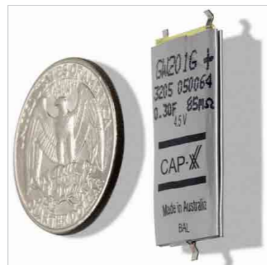
Figure 2: Designers needing to accommodate space-constrained designs might consider thin prismatic supercapacitors
