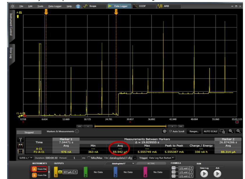
Figure 4: The Agilent 14585A Control and Analysis Software can be used to determine battery runtime.
