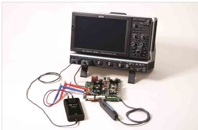
Figure 4: High-voltage differential probes handle common-mode voltages up to 1 kVRMS.
