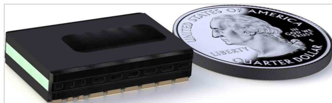
Figure 4: Advanced packaging technologies, such as Vicor's ChiP, support symmetrical thermal designs exploiting top- and bottom-side cooling.
