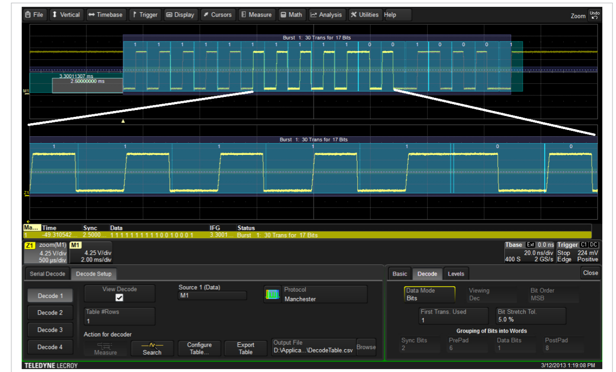
Figure 2: Verifying correct bit-level decode with a zoomed view
