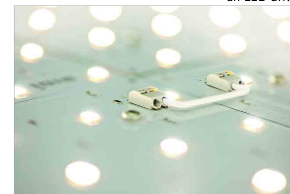
Figure 2: The compact size and light color reduce shadowing in an LED application
