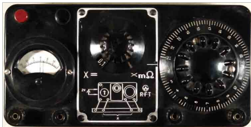
Figure 2: An early Kelvin bridge for making accurate resistance measurements of very low-ohm resistors supply current through resistor X, while the inner leads isolate the measuring circuit. It is easier to see the Kelvin sensing principle in Figure 3.
