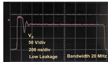
Figure 6: Secondary diode voltage for low-leakage transformer design with 20 MHz bandwidth rather than 200 MHz. Note the turn-on spike is no longer visible.
