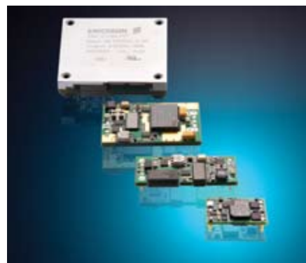
Caption: Ericsson bricks have reduced in size from half, quarter, eighth, down to sixteenth, all of similar power rating.
