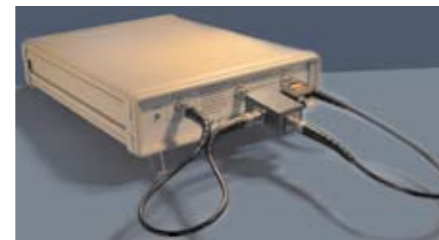
Figure 4: Impedance measurement test setup using the AP200 frequency response analyzer.
