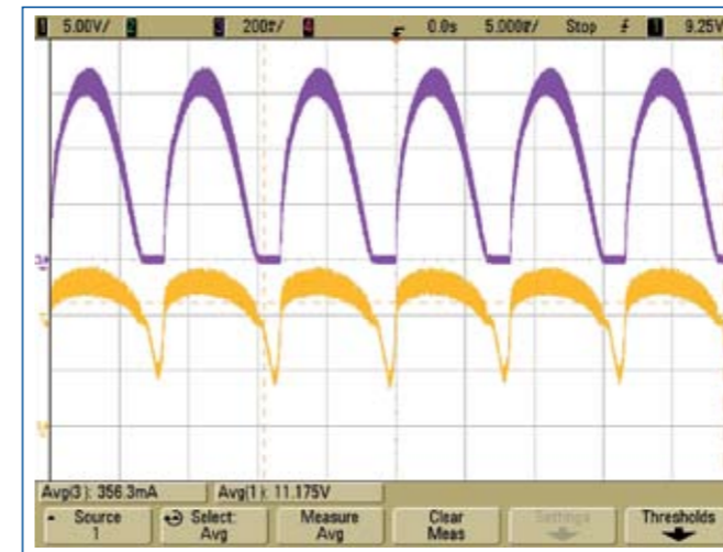
Figure 2: 120Hz AC LED current and voltage waveforms delivering ~4W of LED power.
