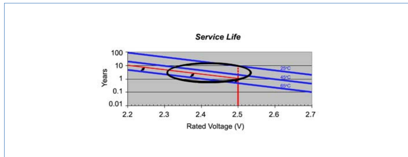
Fig. 1: Life-time of WIMA SuperCapacitors at 2.5V.
