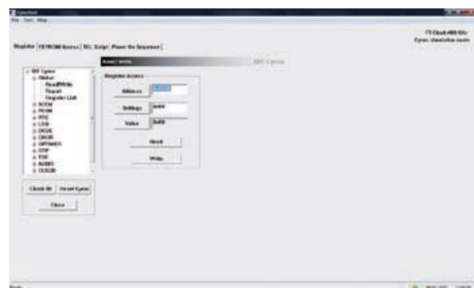
The GUI allows the user to quickly and easily monitor and change P95020 register settings
