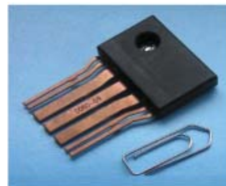
Figure 7: eupec 180 A / 75 V MOSFET half bridge module "CarPACK".
