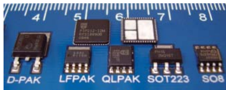
Figure 6: The PIP212-12M that contains two MOSFETs and a driver IC inside a compact 8mm x 8mm package (shown front and back) compared to discrete power packages.
