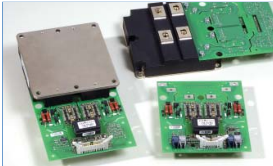
Figure 2. Plug&Play driver boards for 140x130mm dual module with electrical and fiber-optic interface.
