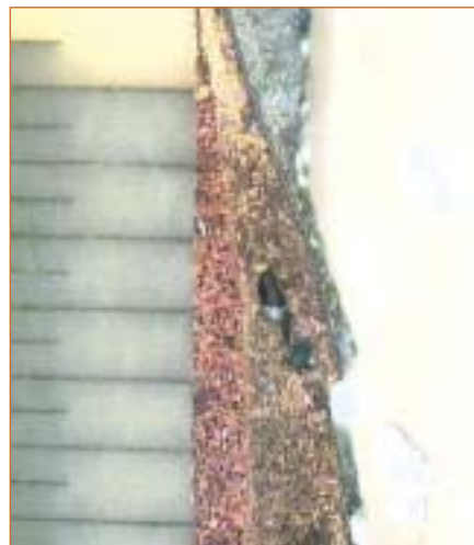
Figure 2. Flexitem soft-termination MLCC exhibiting tearing of the epoxy layer at the edge of the device.
