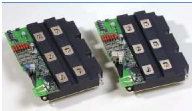
Figure 8. 1SD536F2, Plug&Play driver with di/dt feedback for 2400A and 3600A single switch IGBTs.
