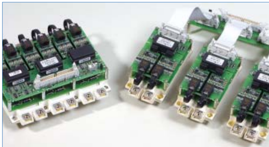
Figure 3. Plug&Play driver solutions for EconoPACK+ and EconoDUAL+ module.
