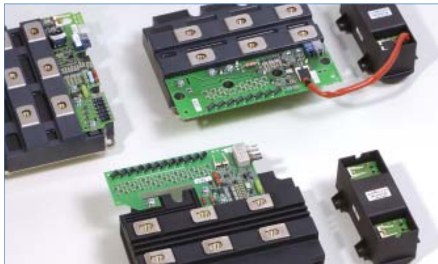
Figure 4. Plug&Play driver solutions for high-voltage IGBTs (3300V, 4500V and 6500V reverse voltage).
