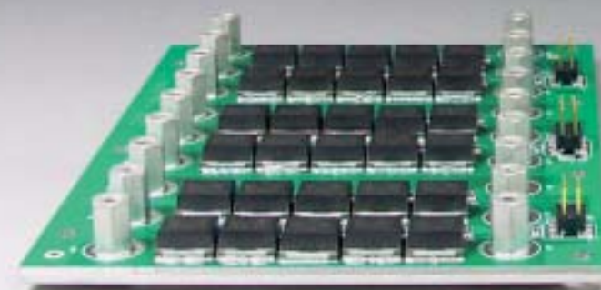
ACTUAL POWER BOARD (18) parts of hardware (30) FETs on (1) T-Clad board
