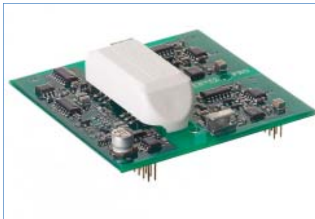
Figure 3. SKYPER 32 PRO core driver is incorporated into each cube.
