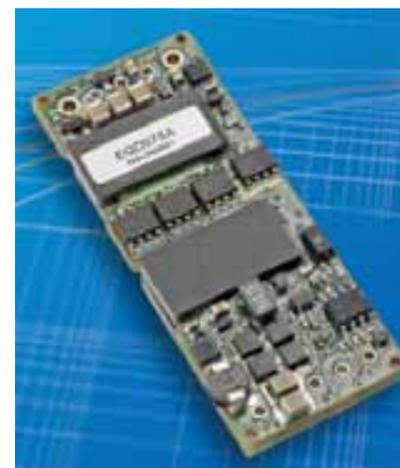
Tyco Electronics Power Systems announced the release of its EQD075A and EQD020A0F series DC-DC converters, part of a new generation of open-frame DC/DC power modules designed for UMTS and CDMA base stations and wireless IP routers applications. These
