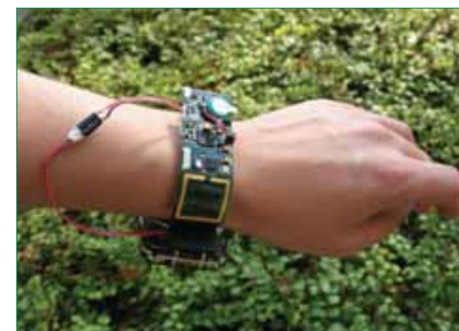
Figure 3b. Electronic modules, mounted on a watchstrap.
