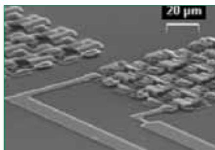
Figure 4. A corner of the chip containing about 2500 poly-SiGe thermocouples forming a thermopile before etching the rim.
