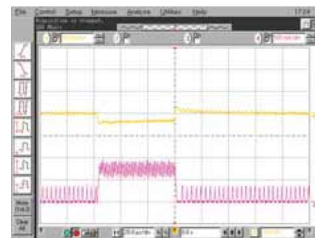
Figure 4. Larger output capacitor and larger feedforward capacitor. Vin=3.8V, Vout=1.8V, Iout=80mA .. 720mA .. 80mA, Cff=220pF, Cout=2 x 22uF. Channel1: output voltage, Channel 4: inductor current.
