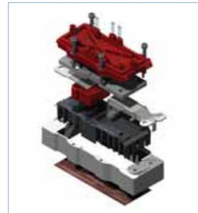
Figure 2. Exploded view of the IGBT halfbridge.
