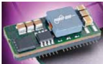
Power-One announces the availability of its 15-amp ZY1015 No-Bus Point-Of-Load (POL) converter. Featuring a low-profile horizontally-mounted package, this hardware-configurable digital POL provides sophisticated power management capabilities without the need for programming, external controllers, or
