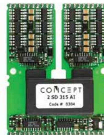
Driver stage for a gate current up to ±15A per channel, stabilized by large ceramic capacitors
