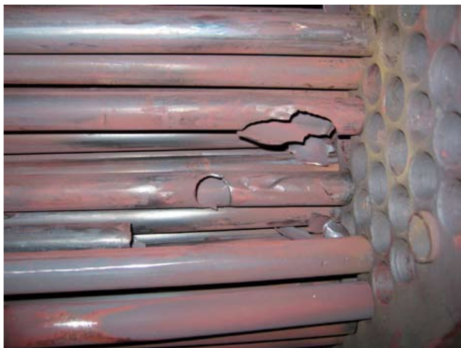
Damage to the desuperheater tubes due to steam impingement.
