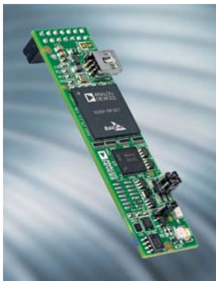
ADI also offers a $150 Blackfin emulator (ADZS-ICE-100B), providing designers with a comprehensive development platform that lowers the cost of entry to the Blackfin BF50x series.
