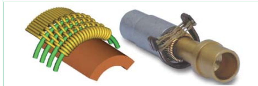
Tribotek connector basic elements showing pure copper wire wrapped around Kevlar tensioning fiber and held in contact to a copper mating pin.
