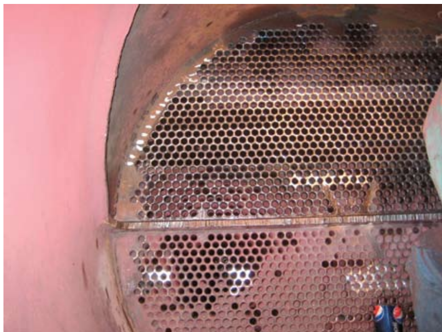
This additional space allowed with the hemi head removed, directly led to a more efficient rebuilding project by providing full access to the tubesheet.
