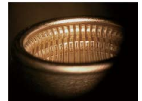
Microphotograph of a PowerBud connector showing two rows of contact fingers. Each finger is formed to allow two points of contact. The illustration shows the details of the first and second conductor rows and the dual contact points on each finger.
