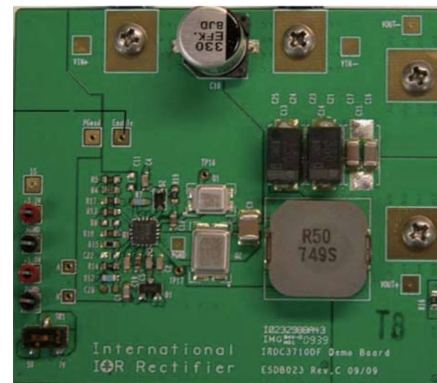
Figure 5: PCB design with IRF6720S and IRF6729M DirectFET MOSFETs.
