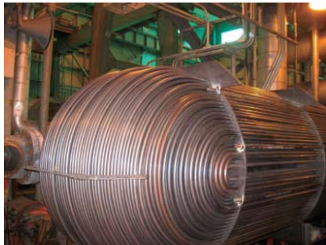
APS undertook the rebuilding project, utilizing its ASME Code shop and 50 certified and trained heat exchanger technicians, code welders, as well as their NDE staff. The work was completed per code, per insurance regulations within a scheduled four week outage.
