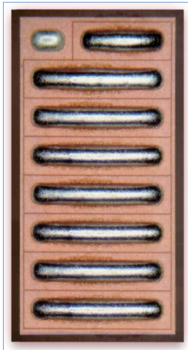
Figure 5: Topside view of a flip chip GaNpowIR device.
