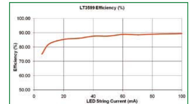
(b) LT3599 Efficiency vs. LED Current Temperature
