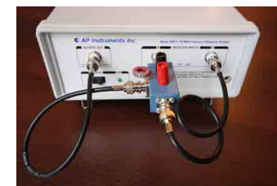
Fig. 6: Photograph of magnetics test setup with AP300 Analyzer.
