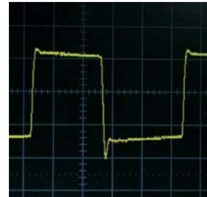
Figure 2: Gate Drive Waveforms with Damaged Gate
