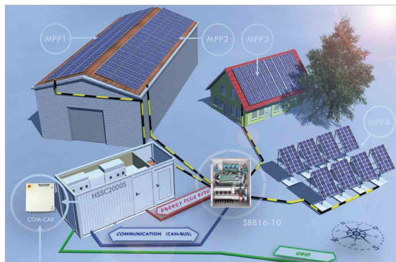
Figure 1: System overview: Container with 2 x 1-MW central inverter and MV transformer, String Booster Box (one of up to 24) and four PV module arrangements that require individual MPP-tracking.
