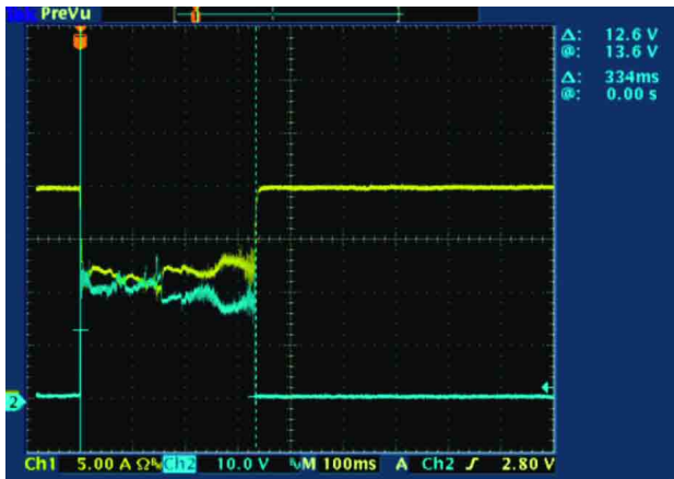
Figure 4a Response curves for a simple bimetal protector at a rated voltage of 24 V and 20 A. The time scale is 200 μs/div; vertical scales are 5 V (blue) and 5 A (yellow) per division, respectively.
