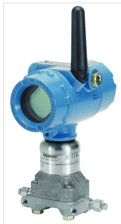
Figure 1: Emerson Rosemount's 3051S series wireless instrumentation exemplifies the benefits WSN brings to industrial applications: It can reduce total installation costs by 45% and total deployment time by as much as 75%, eliminating design and installation time and cost associated with wiring, conduit, cable trays, and junction boxes. joining a $1.5 billion chip company with global presence, the acquisition has enabled
