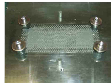
Figure 3: Glass pane with TIM applied mounted to a heat sink
