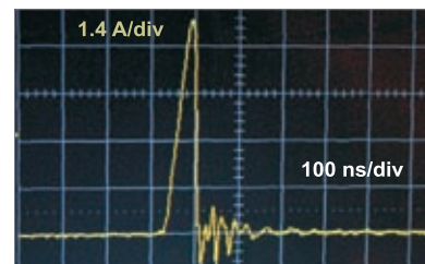
Figure 5: Current sense waveform with high-line voltage input and short-circuit on output. Notice that the current pulse is reduced to just 100 ns. When this current signal exceeds a second current limit threshold, soft-start is reinitiated, and the converter enters a burst mode of operation at low frequency, protecting the semiconductors from overstress.
