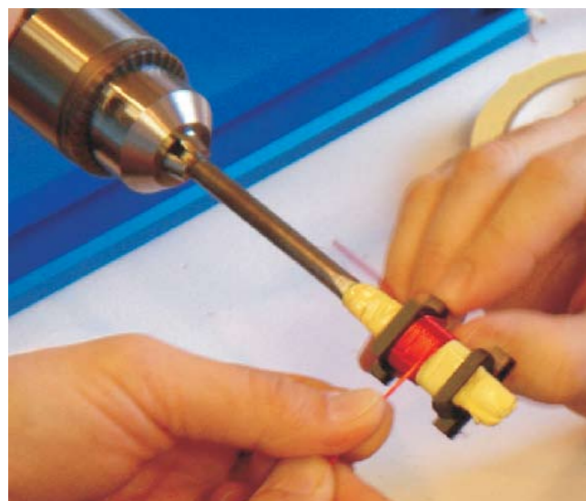
Figure 1: Building custom magnetics in our design workshop.
