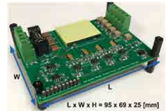
Figure 2: The prototype of a 400W DC/DC MPPT, Non-Inverting Buck Boost (NIBB) converter
