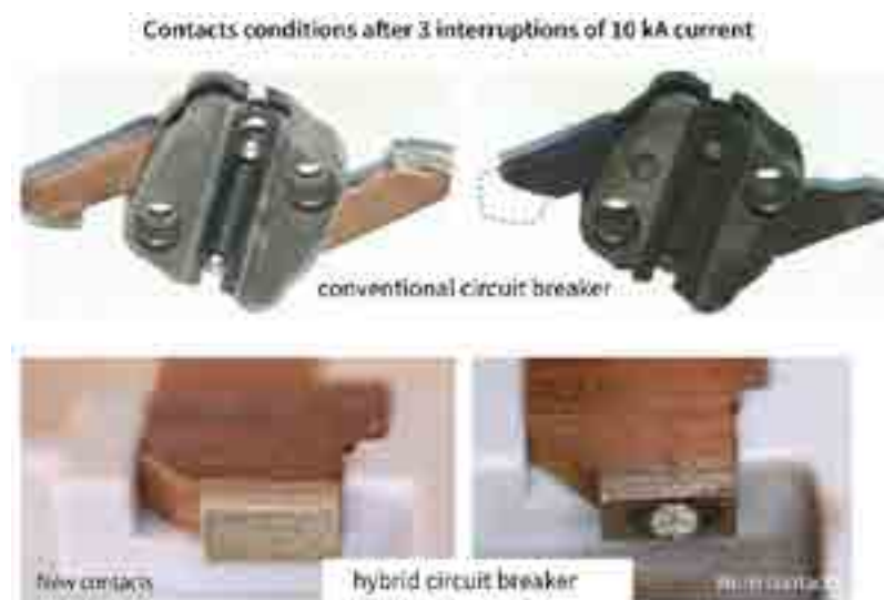
Figure 1: Contact wear in an electromechanical relay (courtesy of Eaton Corporation)
