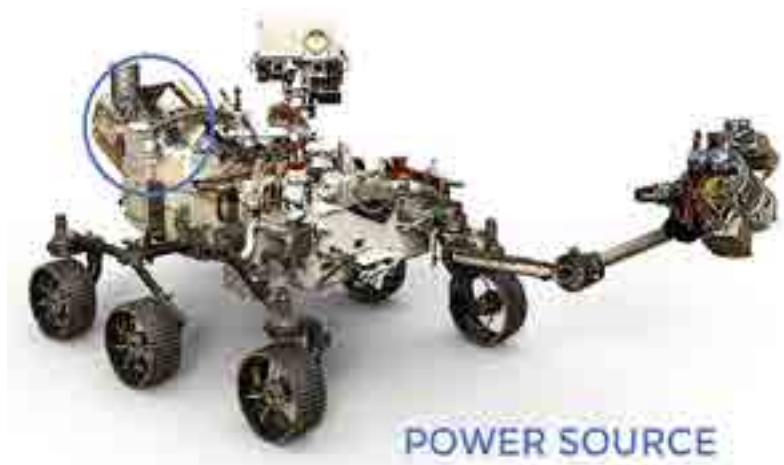
Figure 6: Mars2020 Rover MMRTG power source circled in blue (Image courtesy of NASA)
