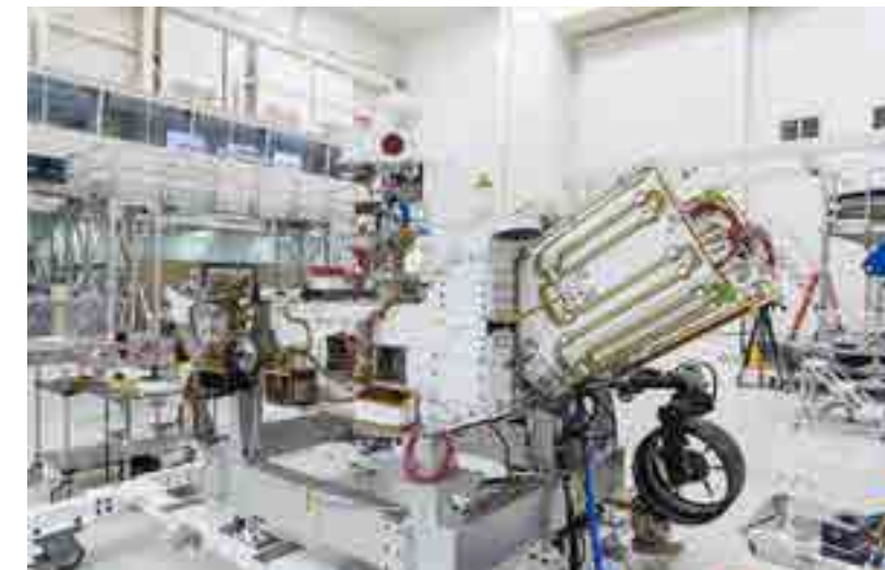
Figure 5: Solar energy powers the Mars 2020 spacecraft during its 9 month journey to Mars, but while on the Mars surface, the MMRTG will be the prime source and heat pumps need to be used as well due to the extreme temperature conditions. (Image courtesy of NASA)
