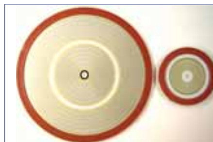
Figure 2. Cathode side of Ø91mm (left) and Ø38mm (right) 4.5kV IGCT wafers.
