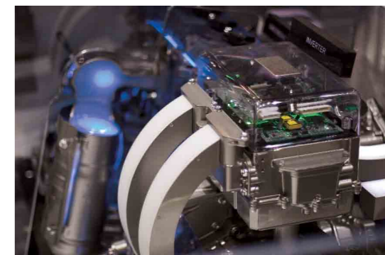
Figure 1: Micro-inverters convert direct current from individual solar panels into alternating current for the electric grid.
