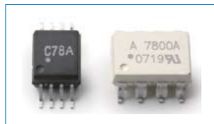
Figure 4: SSO-8 package (left), 30 percent smaller footprint vs. DIP-8 package.
